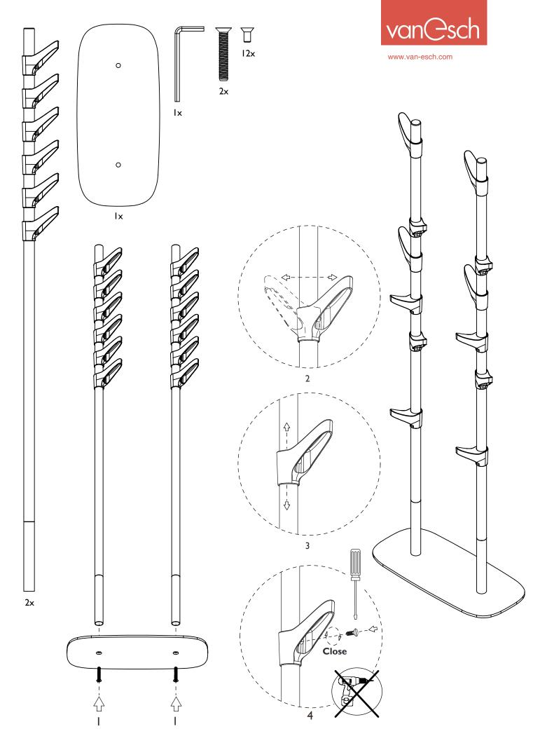
To avoid damage: before adjusting the hooks, make sure the plastic bolts are sufficiently unscrewed.
