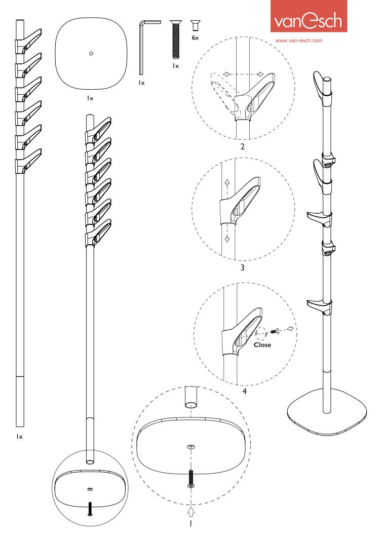
To avoid damage: before adjusting the hooks, make sure the plastic bolts are sufficiently unscrewed. **SLIDE GI WOOD**
